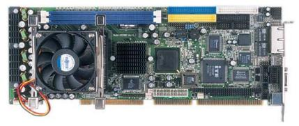
The CPBH is an Intel<sup>®</sup> 82865GV/82801EB chipset-based board designed for PICMG Bus PGA 478 Intel<sup>®</sup> Pentium<sup>®</sup> 4 CPU with speed of up to 3.2GHz CPU. The combination of these features makes the CPBH an ideal all-in-one industrial single board computer. Additional features include an enhanced I/O with CRT/LVDS Panel, TV-Out, dual Giga LAN, audio, serial ATA, 4 COM port interface, and more.
